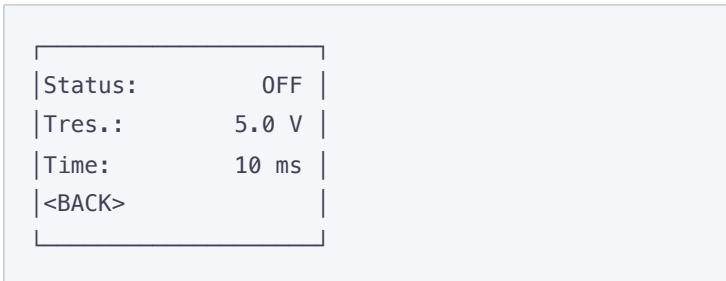
Figure D.6.5 – Screen of setting the Upper and Lower thresholds of event
