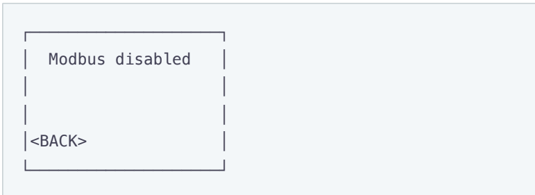
Figure D.8.1 – Screen of switching on and switching off of Modbus TCP server
