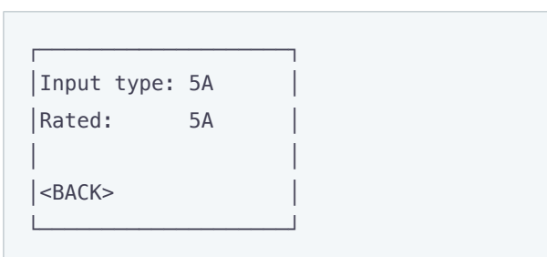
Figure D.2.2 – Screen of setting of current transformer rated
