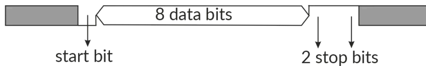
Figure 5 – Byte format without parity control (2 stop bits)
