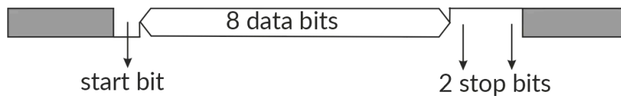
Figure 5 – Byte format without parity control (2 stop bits)
