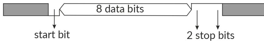
Figure 5 – Byte format without parity control (2 stop bits)
