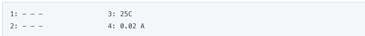
Figure 5.5 – Showing the state of inputs on the display (sensors 1 and 2 are disconnected, a sensor of temperature 3 – 25°C, a sensor of current 4 – 0.02 A)
